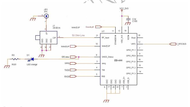
[Note 1]: VRTC (pin#12) could connect to 3.3V DC power supply or battery directly. (EB-600)
