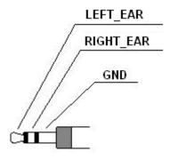
Or using the PL602 connector where the pin-out is the following:
