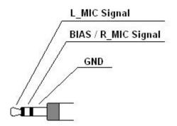
Or using the PL306 connector where the pin-out is the following:
