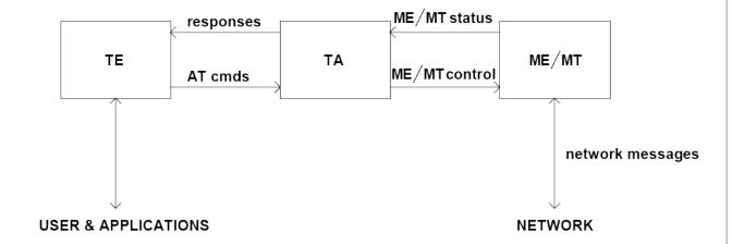
TELIT MODULEs physical implementation of this abstract architecture integrates the TA under the ME cover, and implements the TE as a separate entity.
