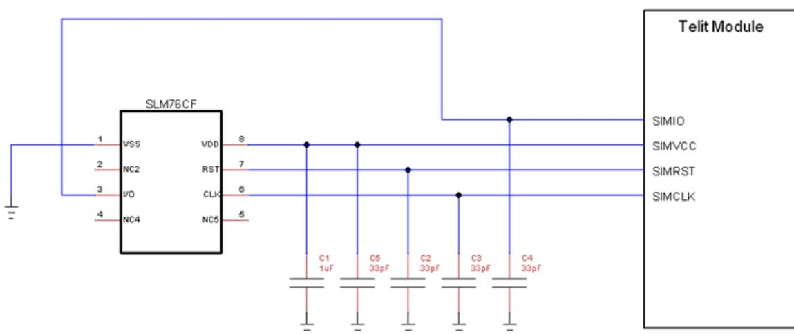
Figure 6-1 SIM On Chip connection
