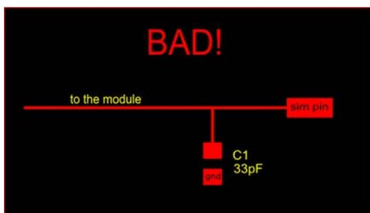
Figure 3-1 PCB Layout 1
