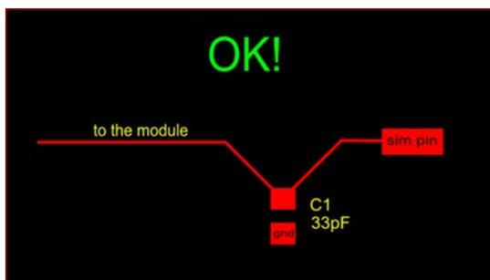
Figure 3-3 PCB Layout 3
