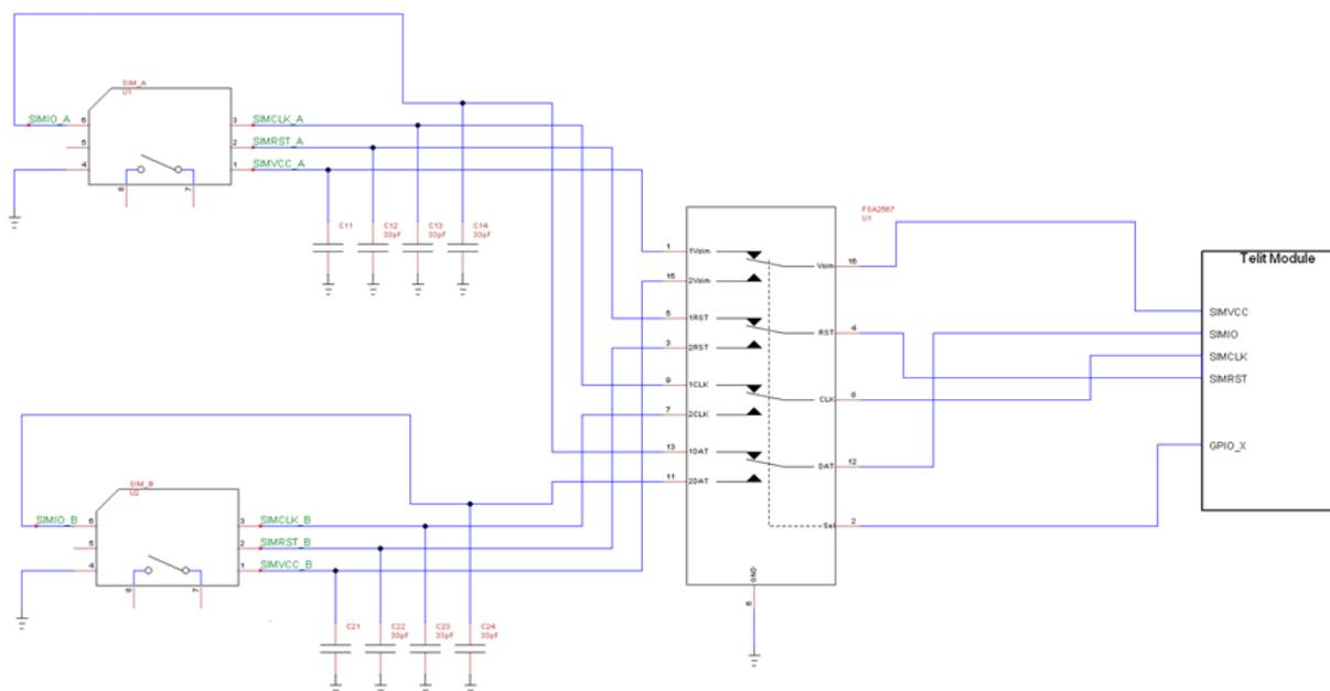
Figure 5-2 switch with a low Ron channel for SIMVCC
