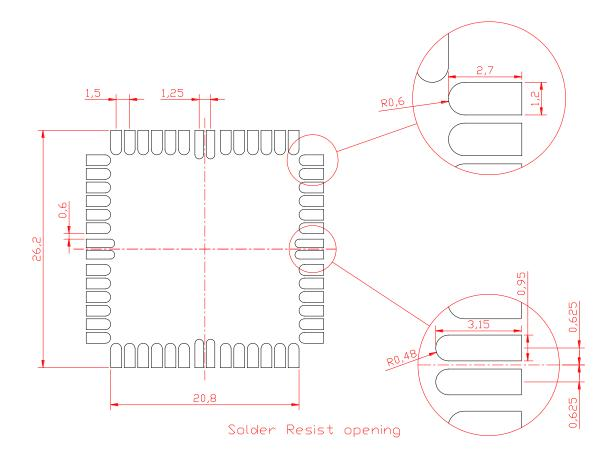
In order to easily rework the NL865H2 is suggested to consider on the application a 1.5 mm placement inhibit area around the module.
