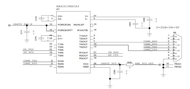
The example is done with a MAXIM MAX3238 Transceiver that could accept supply voltages of 3.3V DC.
