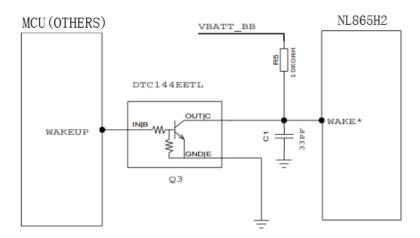
The resistor and capacitance in Figure are only the recommended value and they need to be tuned according to the specific customer's application.
