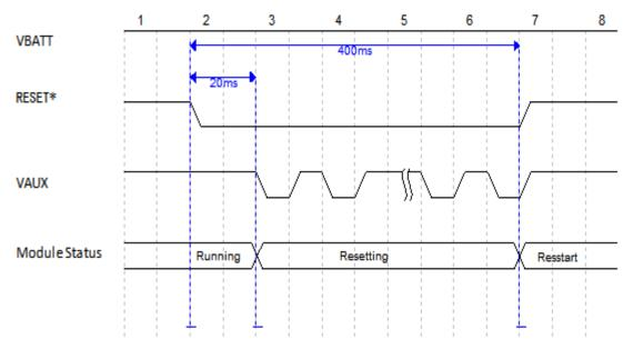
The RST timing is shown in the following figure below:
