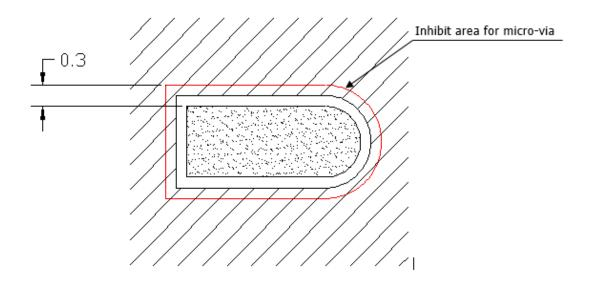
Holes in pad are allowed only for blind holes and not for through holes. Recommendations for PCB pad surfaces:
