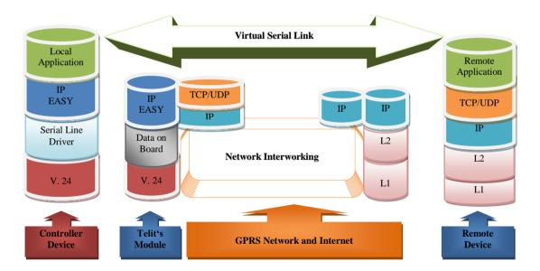
This particular implementation allows to the devices interfacing to the Telit GE866-QUAD module the use of the GPRS and Internet packet service without the need to have an internal TCP/IP stack since this function is embedded in the module.
